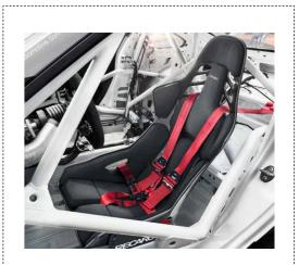
Fasten your seat belts! The RECARO Podium CF can be used with all standard belt systems for road and track: 3-, 4-, 5- or 6-point belts.
