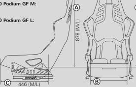
Comfort measurements: A: Seat height B: Seat width C: Seat depth Dimensions in mm, all dimensions +/- 10 mm
