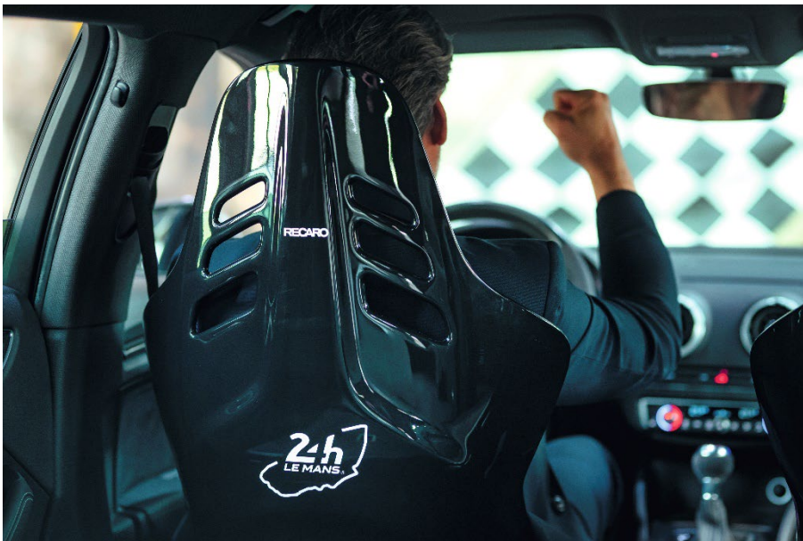
The Podium GF combines high-strength, ultra-lightweight high-tech foam in the shell core with a front and rear shell made of glass-fiber-reinforced plastic (GFRP). Source: Recaro Automotive
